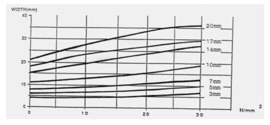
**Chart 4**Gasket thickness in relation to clamping pressure.
