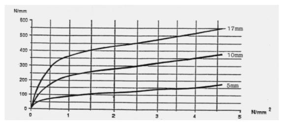
**Chart 3**Gasket width in relation to clamping pressure.
